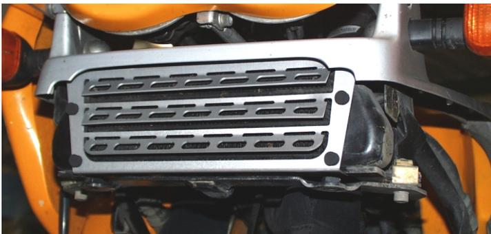
Oil Cooler Protection is simply slid on the oil cooler. Rotating of the Oil Cooler Protection is not possible without use of force.
